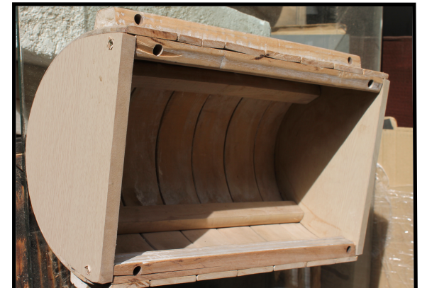
I used a 2x2 (1.5" by 1.5") to gage the ht. from the bottom of the lid. I secured the crossmembers on the inside walls with screws that I had salvaged earlier...
