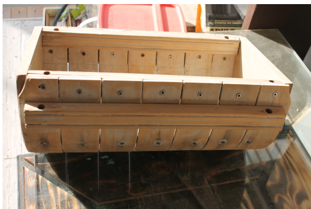
Here, there are 4 cross members attached to Lid. The inside is flush, and the outside is approx. 1.5 in. from the bottom of the exposed slats.
