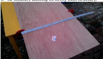
4. Measure, mark, clamp and drill all corners at 3/4" x 3/8" with 1/8" drill bit.
