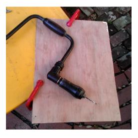
5. When ready, glue support beams, align tabletop, clamp and attach with screws.
