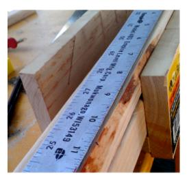
1. We'll begin with the legs. Measure lumber with yardstick and mark the pencil then use the triangle to make straight line off the straight edge. Make the marking all around the lumber, use triangle for accuracy.
