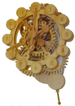
Synchronicity is a wood gear clock with a unique drive mechanism – a microcontroller-regulated electromagnetic pendulum drive. This document contains listings of the microcontroller software. The clock itself is documented in an Instructable at http://www.instructables.com/id/A-wood-gear-clock-with-a-unique-drive-mechanism/.
