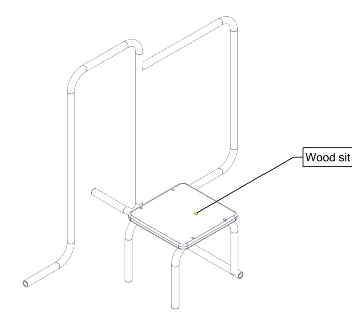
Cut a piece of wood measuring 25 cm x 25 cm and 20 mm thick. Pre-drill holes in the wood for the final connection to the frame. Use self-tapping screws and carefully screw the seat to the frame.
