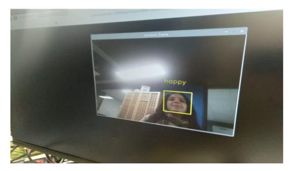
we are going to implement an Emotion Recognition System or a Facial Expression Recognition System on a Raspberry Pi. We are going to apply a pre-trained model to recognize the facial expression of a person from a real-time video stream. The "FER2013" dataset is used to train the model with the help of a VGG-like Convolutional Neural Network (CNN).
