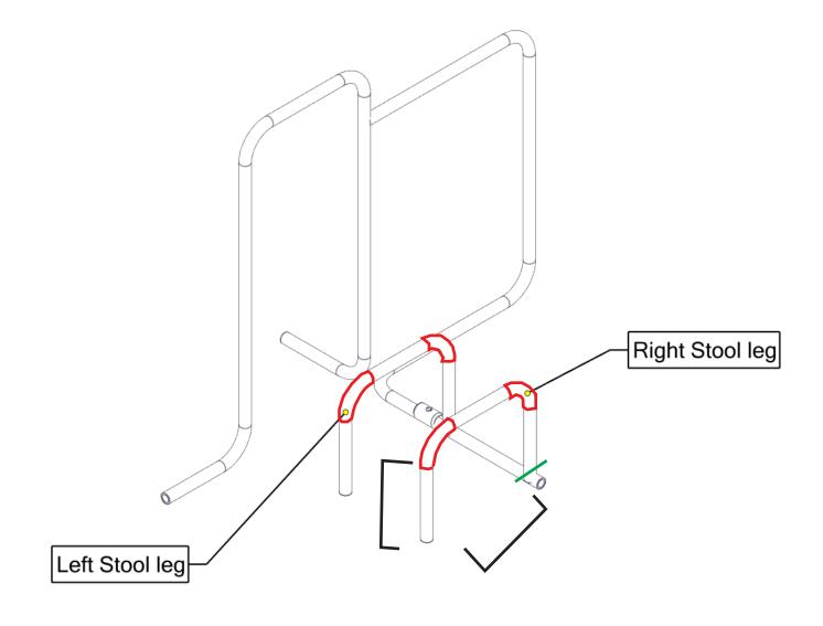
Bend the pipes so that they complete a half shape as shown in the diagram. After bending, cut one end to a depth of 22 mm. Then weld the **cut** end to the pipe as shown in the diagram. The distance between the pipes is 17 cm.
