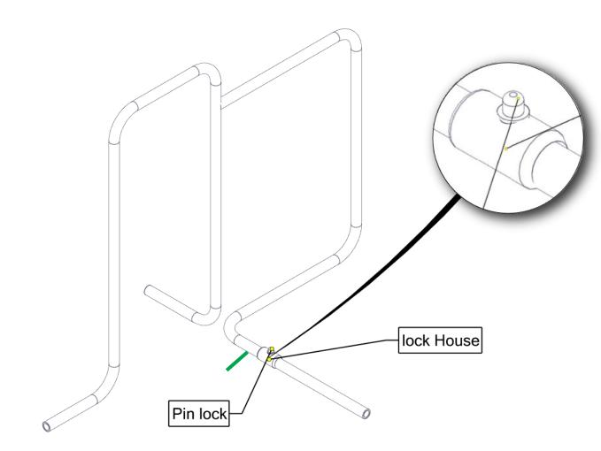
Take a 25 mm diameter pipe and cut a 65 mm long piece from it. Drill a 10 mm diameter hole 23 mm from the marked end.
