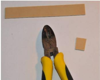
A pair of large diagonal cutters is very well suited to cutting the PCB stock.
