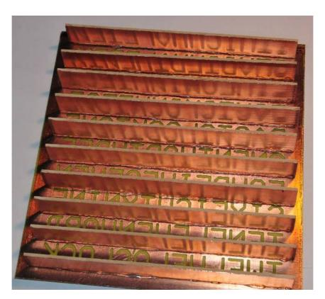
Next, we need to glue in the vertical baffles – these are cut of the remaining baffle pieces.
