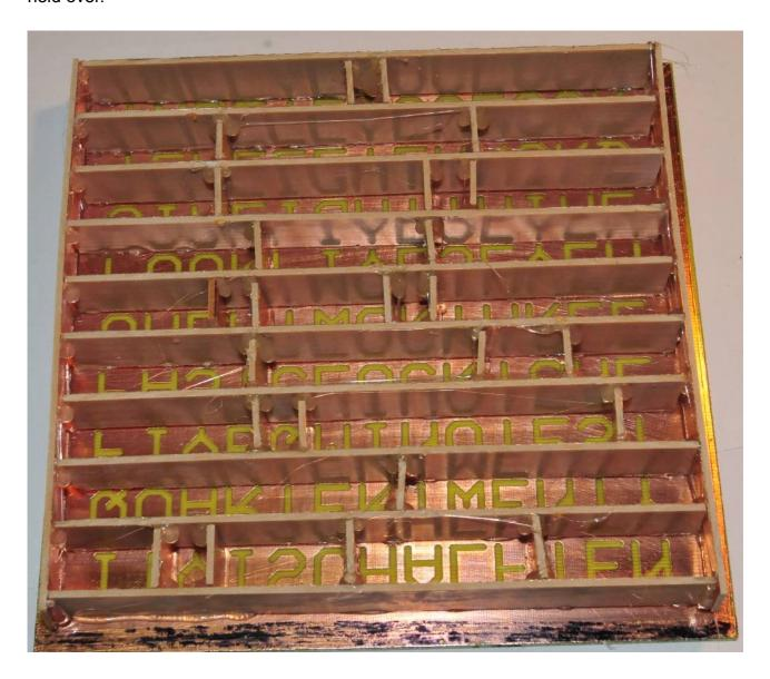
Start by running a bead of glue along the baffle edge, then run a bead up every second horizontal. Quickly position the edge, and hold it till the glue dries.
