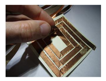
When you are ready to place the last piece of copper tape, put down a strip of masking tape over the copper tape already on the paper.
