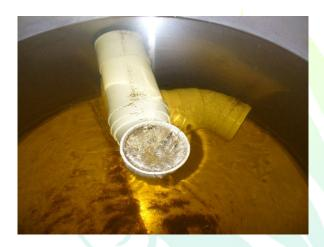
Figure 1: A swirl sedimentation tank showing the tangential inlet (bottom of the tank) and the solids being directed to the centre bottom of the tank. The outlet is at the water surface or centre of the picture.
