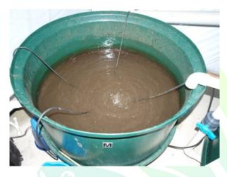
Figure 5: A simple "off line" solids mineralisation tank showing aeration. The pipe and valve at the right is the solids drain from the sedimentation tank to the mineralisation tank.
