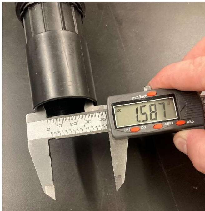
7. Measure the inside diameter (in inches) of your vacuum hose using calipers. Subtract this value by 0.02 inches and divide it by two.
