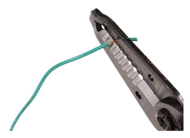
To do this, strip the insulation off of the ends of two pieces of stranded wire using your wire stripper.
