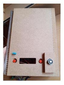
Attach the side and top by screwing them together and don't forget to put wood glue in between. The component plank will not fit because the gas spring is in the way. Somehow I needed ventilation. I attached a grid of 34,0 x 2,5 cm on the left to the top plank.I still had to reach my RPi for another project, so I didn't screw it down to the outside of the case. I made two support blocks on which the inner shelves can lie.
