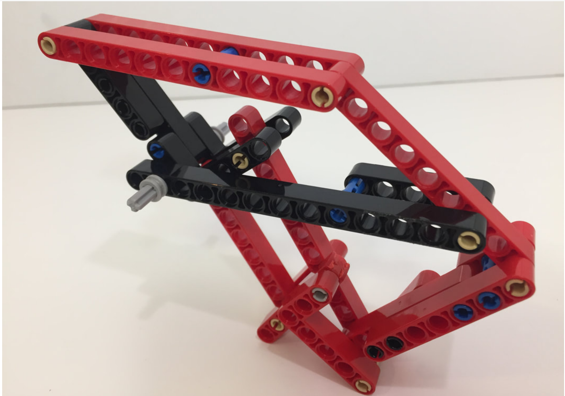
TrotBot's Leg Mechanism with Retractable Toes
