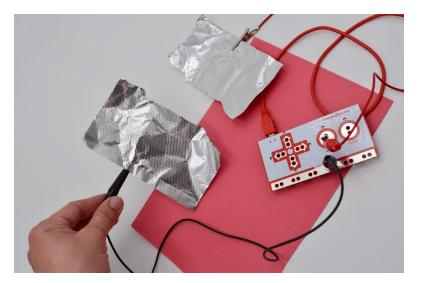
Incomplete Circuit: Electrons cannot flow...
