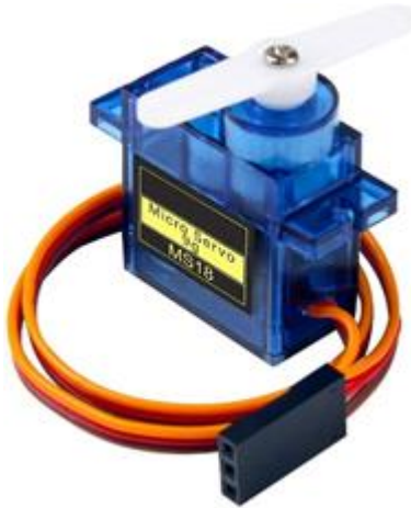
Figure 10- Image of a Micro Servo 9g MS 18 taken from Amazon (It is the same model as the Micro servo SG 90 and it have the same features). This motor is programmed writing angles and it has a maximum rotation of 180°.
