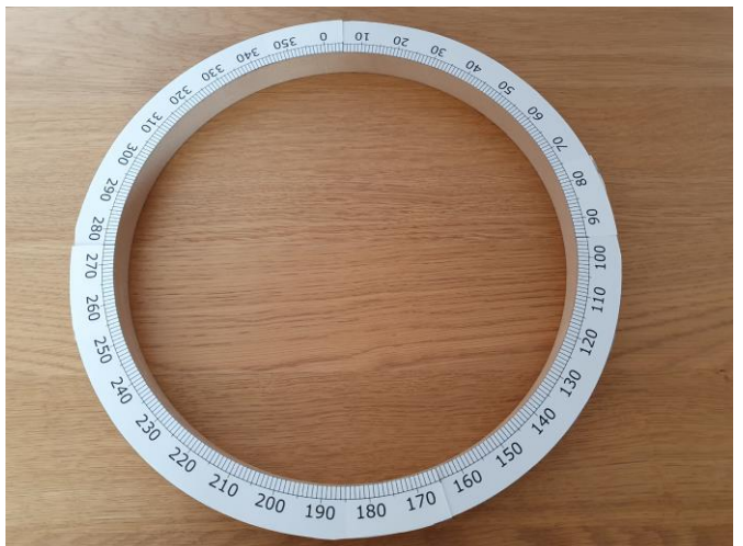
Printed Scale Trimmed and laid on Annular Ring – Approx 15° overlaps
