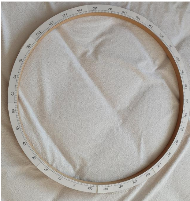
Printed Scale Trimmed and laid on Annular Ring – Approx 10° overlaps
