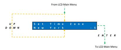
Press *UP* & *DOWN* buttons to increment & decrement the Time Zone by one hour, a major city and offset from UTC is displayed for each Time Zone. Press *ENTER* button to select the Time Zone and return to the LCD Main Menu
