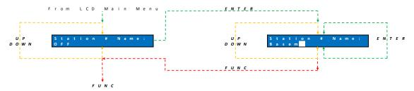
Press *UP & DOWN* buttons to cycle through the Station Menu
