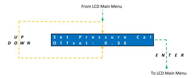
Press **UP** & **DOWN** buttons to increment & decrement the offset in steps of 0.01 inHg Press **ENTER** button to save the offset and return to the LCD Main Menu
