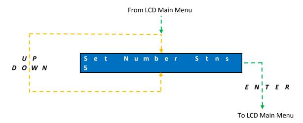
Press **UP** & **DOWN** buttons to increment & decrement the number of active stations, respectively Press **ENTER** button to return to the LCD Main Menu
