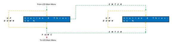
Press *UP* & *DOWN* buttons to cycle through the Station Menu showing humidity threshold for each station Press *ENTER* button once to edit humidity threshold for the selected station Press *FUNC* button to return to the LCD Main Menu from the Station Menu
