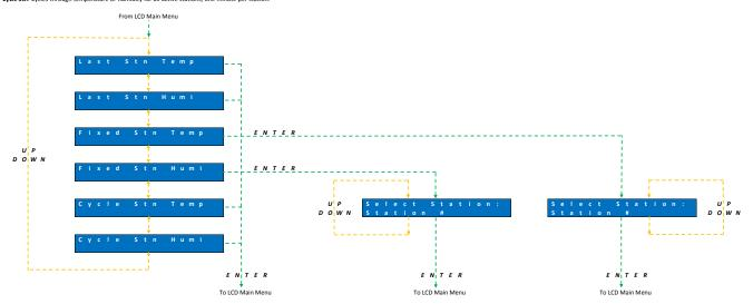
Press UP & DOWN buttons to cycle through six display modes
