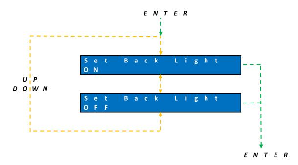
Press **UP** & **DOWN** buttons to toggle back light setting ON and OFF
