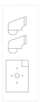
Motor mount /Control horns 1.5mm thick Hobby Plywood
