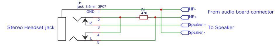
Clever schematic to adapt mono audio output to stereo headset with attenuat - When no headset connected, R1 is bypassed and speaker receives full power - When headset is inserted, speaker is disconnected and R1 is attenuating pow
