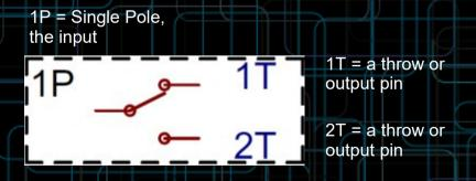
By moving the sliding switch position on the top of the switch you are changing which output pin is connected to the input pin inside the switch.
