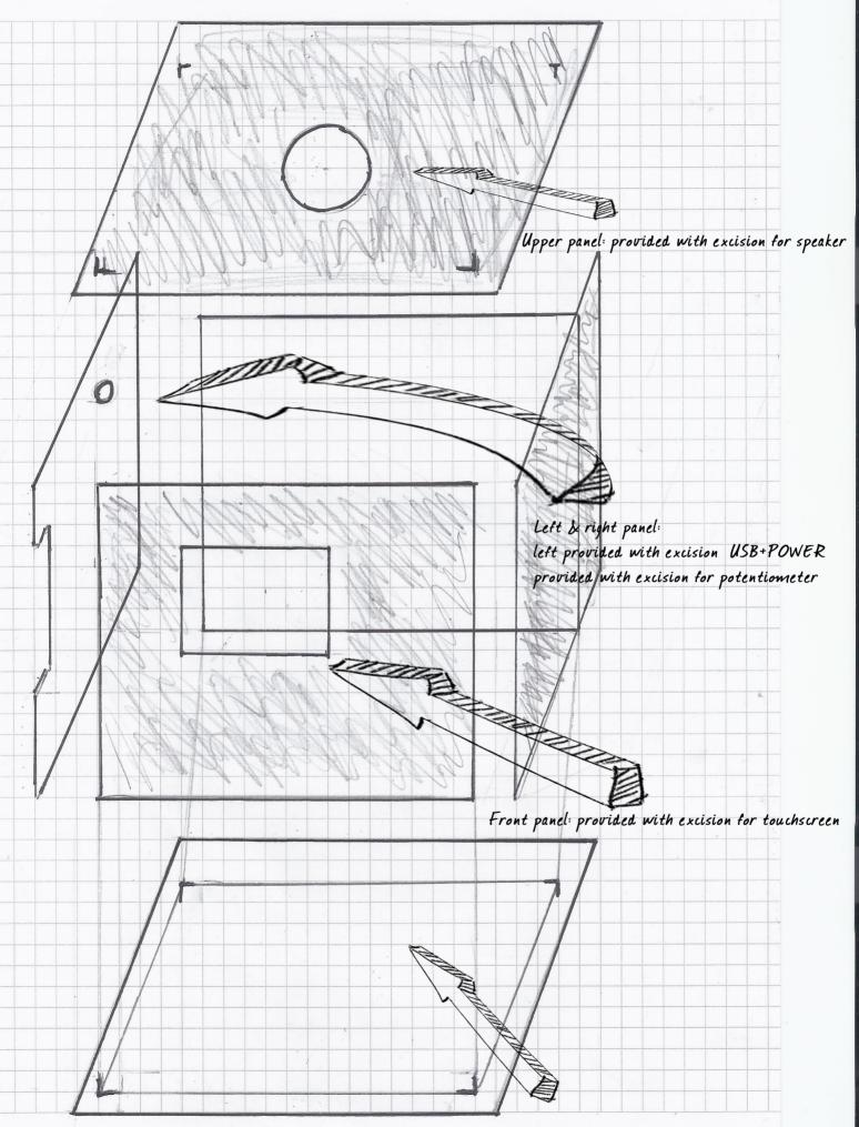
Base panel: for mounting of both side panels + front and back
