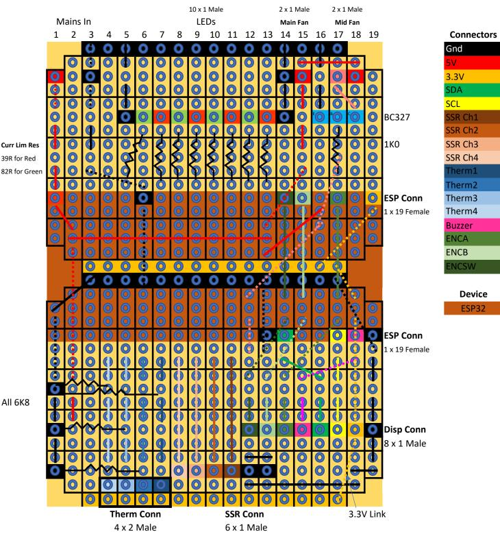
Dotted lines indicate connections on the back of the board Wired connections are only attached at each end!
