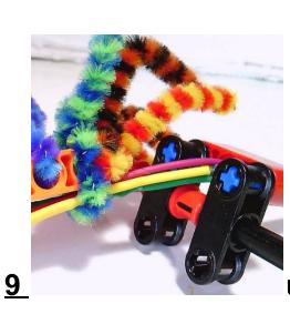
use pipe cleaners to hold wires
