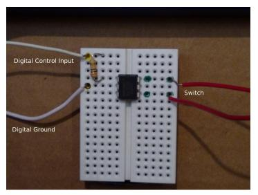
A Clare LCA110 solid state relay chip allows you to switch any low power (battery powered) circuit ON and OFF using the RTBobble Bluefruit. Connect the solid state relay as shown in the diagram. The Digital Control Input is attached to pad A4. The Digital Ground Input is attached to any of the Gnd pads. The switch output connections will replace the switch in your circuit.
