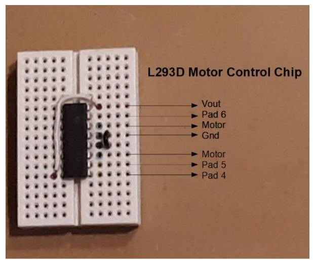
Connect the Circuit Playground Bluefruit's Vout, Ground (Gnd), Pad 4, Pad 5, and Pad 6 to the L293D as shown. Connect the motor to the two pins labeled Motor in the photo. The "+" command will turn the motor ON. The "-" command will turn the motor OFF. "F" will move the motor in the forward direction. "R" will move the motor in the reverse direction. "Z" (Zap) will turn the motor ON for 750 msecs and then turn the motor OFF.
