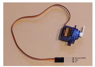
A servo has three wires which are defined as follows:
