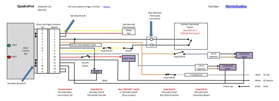
Neutral Wiring "White" The AC Neutral wiring (white wires) is a bit convoluted... and requires the Controller to be in-place to connect everything together.
