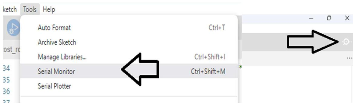
When the ESP32-CAM has been put into programming mode, the serial monitor screen will display the message 'waiting for download'.
