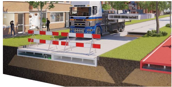
Figure 11: Visualisation PlasticRoad. Source: (PlasticRoad, 2019)
