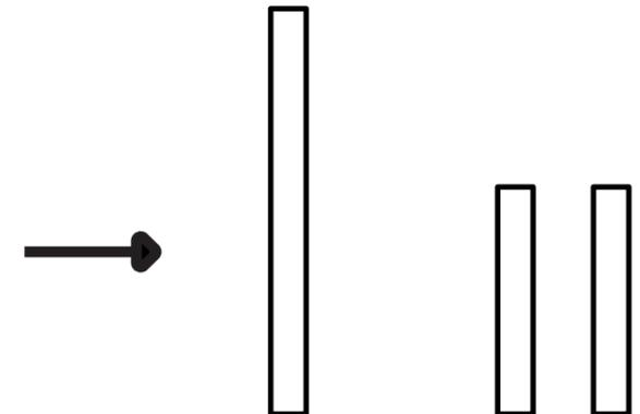
Divide into two parts 60 mm long each, and one part 110 mm long
