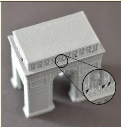
Gaps in Floor Corners
