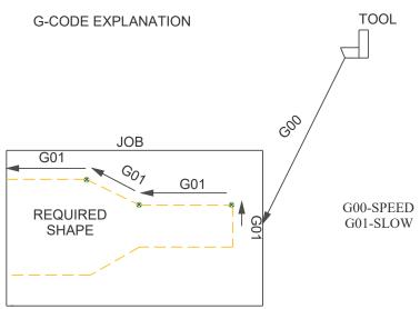
$\otimes$  -represent the points where the tool has to move to get the required shape of the material
