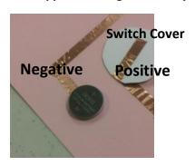
10.) Make sure the copper on the switch lines up to touch the battery when you push on it.
