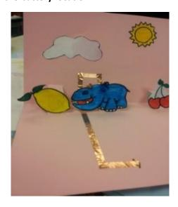
Leave the copper tape a little longer if you are not sure where you want your battery. The circuit works better if the tape is all one piece. Cut 2 two-inch parallel lines through the fold for each pop up. Doing this creates the 'pop-up' effect.
