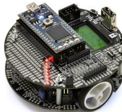
Pololu m3pi robot controlled by an ARM mbed development board.
