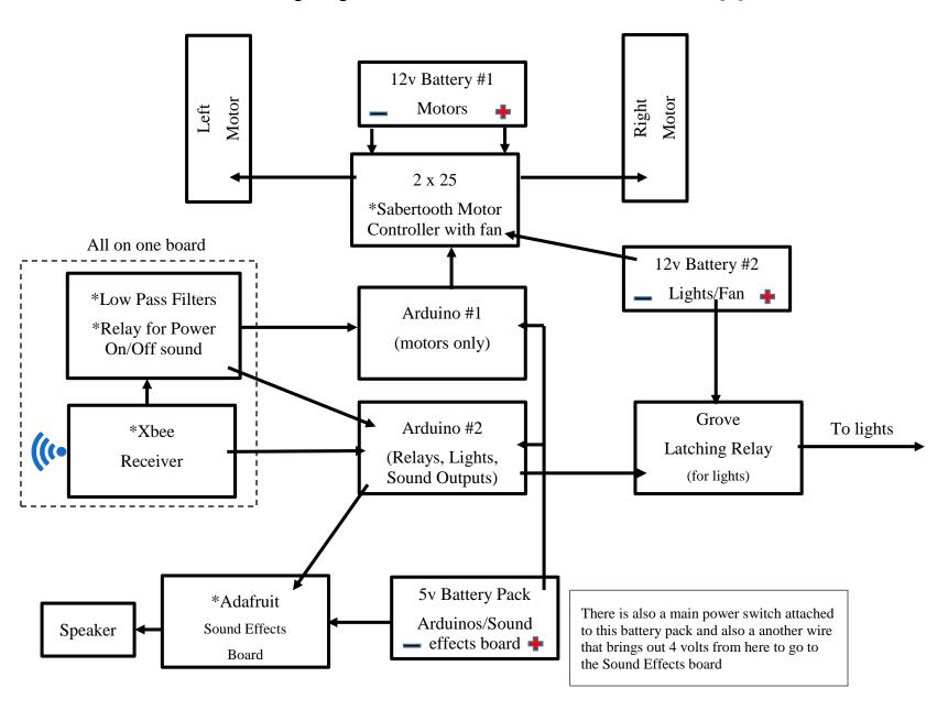
Low pass filters – used to buffer the PWM signals sent out by the Xbee before they enter the Arduino and get converted to servo signals.
