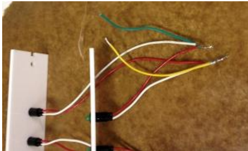
Figure 5-5, The Sunday AM/PM LED Lead Pairs with Pigtail Wires.
