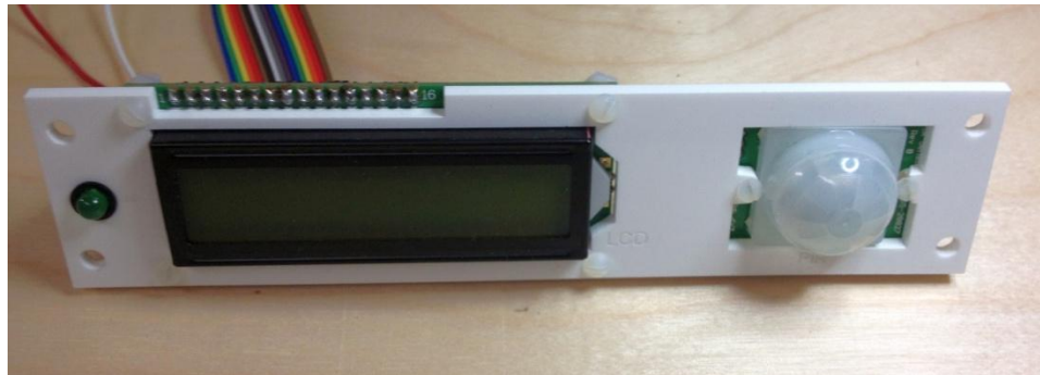
Figure 4-2. Sub panel with parts mounted.
