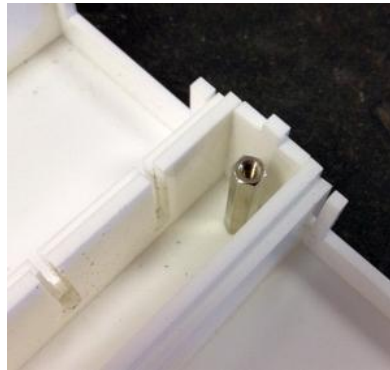
Figure 7-1. One standoff in place. There are four to be installed.
