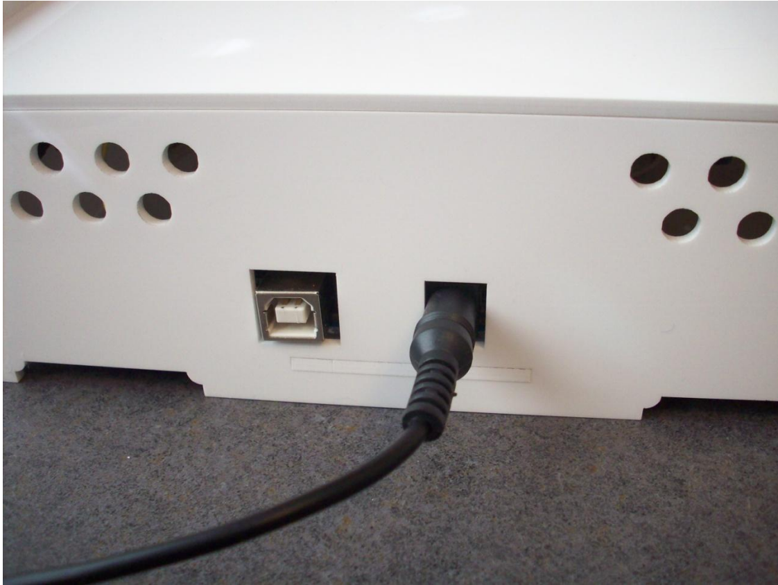
Figure 2-1. Back of Pill Reminder, showing the power supply plugged in.
