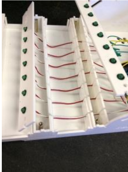
Figure 7-4. PM LED leads are all in place.
