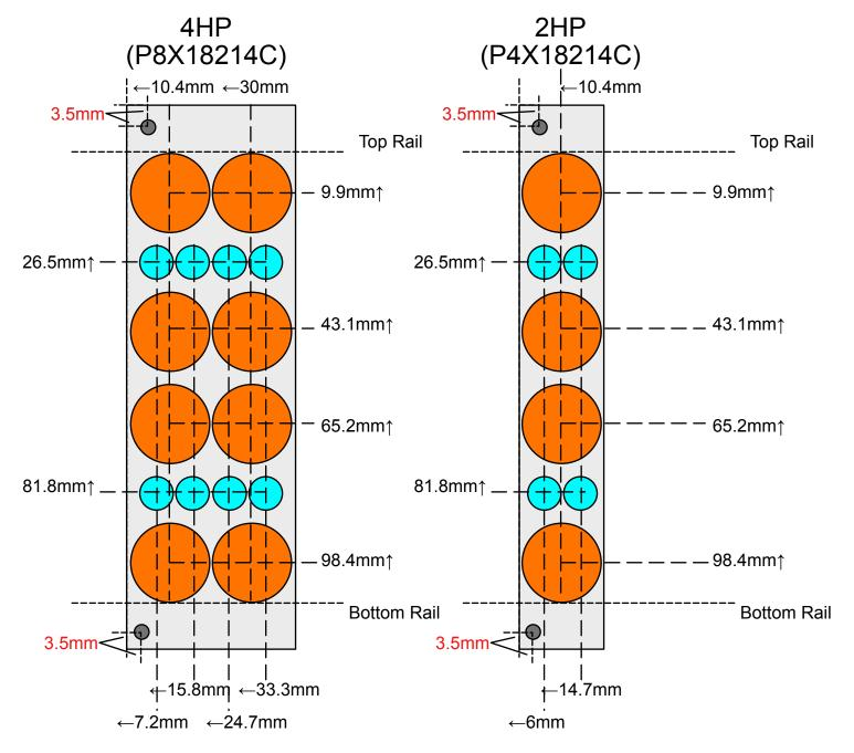
All ↑ measurements are to INSIDE OF TOP RAIL using TipTop Z-Rails. Not guaranteed for all manufacturers-adjust if you need to.
