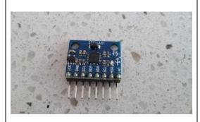
MPU 6050. The MPU 6050 generally is supplied with straight and right angled header pins which need to be soldered on.
