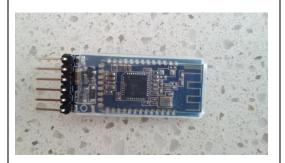
AT09 BLE bluetooth module. You need to configure the baud rate to 115200 (default is 9600). Also you may wish to configure a unique Bluetooth name.
