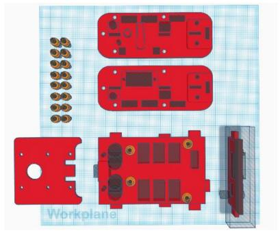
A number of heads are included. These heads can slot into the top of the robot.
