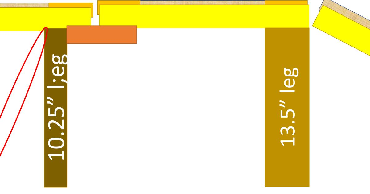
Left is 40wx36l cut down from 54x36. add cut ends to sides for cross support "Pinned" removeable legs at corners. Legs bolted and swing for storage, can have longer legs if back seats are ever fully removed. Middle has transverse mounted 2x6 for legs (removable) that sit on the hard high-ridge line of floor
