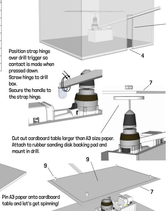
Make a cardboard box 700 x 700 mm and higher than the spinning table to catch paint spray.
