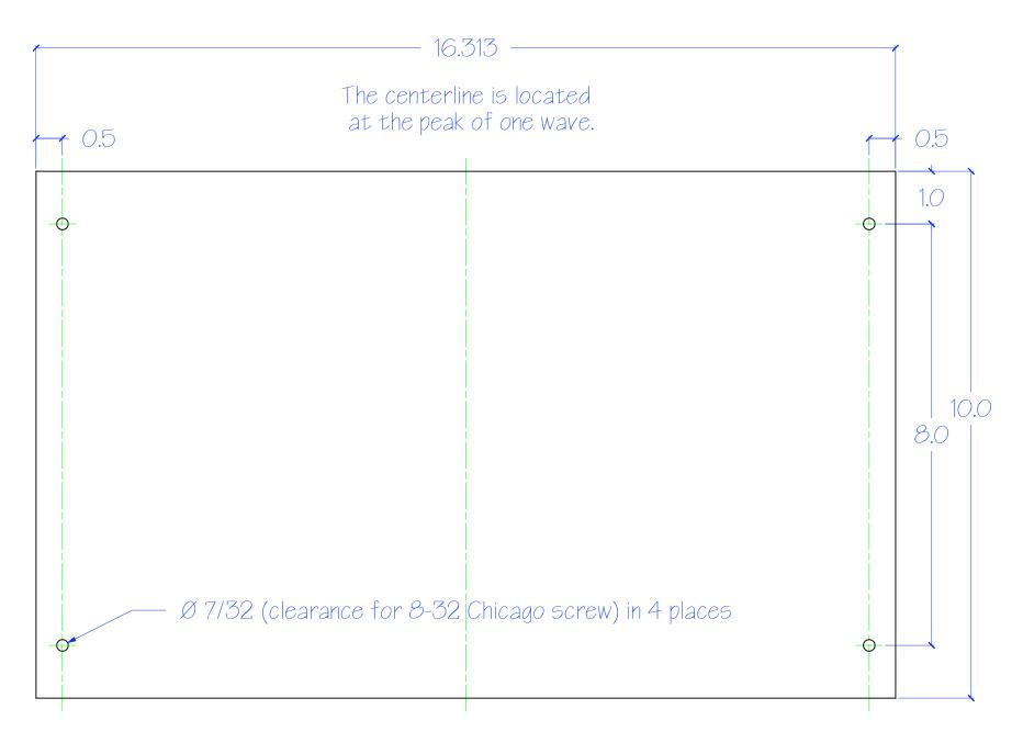
NOTE The width of 16.313 works well for the corrugated sheet with waves repeating every 2.875". If you use something that is different, you may need to modify the width to suit. Fit with the aluminum mounts may be affected.
