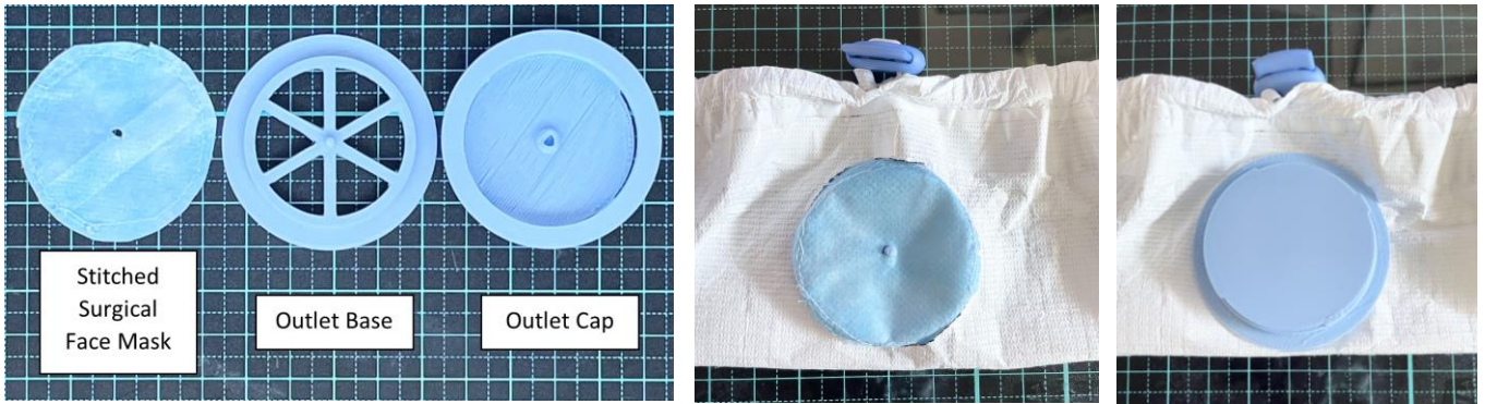
Figure 5: Outlet filtration components (left), components attached (right)
