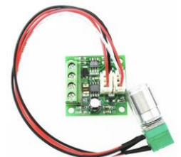
Figure 10: PWM controller and pot-switch
