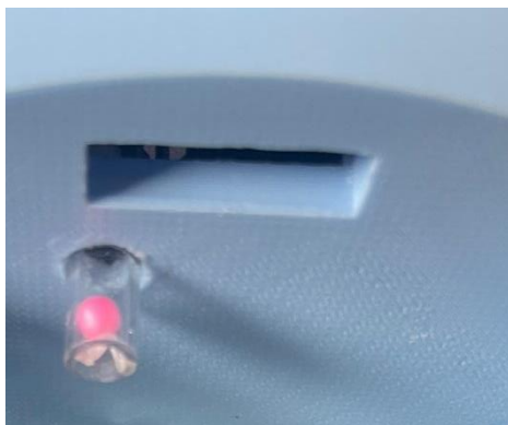
Poor airflow (ball has not risen)
