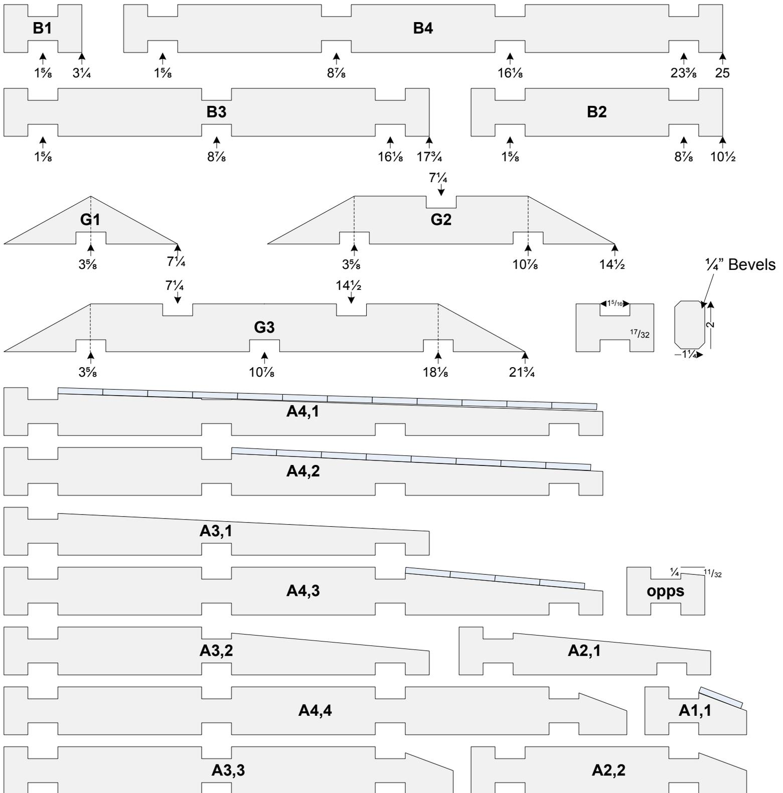
There are four kinds of components; Beams (**Bx**), Gables (**Gx**), Halves (**Hx**), and Awning (**Ax,y**). Halves are just Beams split in half. Awning are made from Beams where the top is beveled  $\frac{1}{4}$ " down from the upper notch to 1" up from the end. (Except when  $x = y$ . Then make the beam 1" longer on the awning side.)
