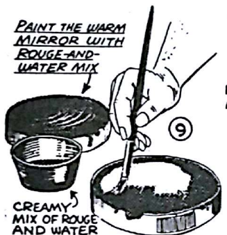
PAINT THE PITCH WITH ROUGE AND WATER. STRIP THE COLLAR AFTER PAINTING
